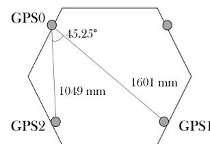
Configuration of the GAP-A payload on the CASSIOPE satellite utilized for array-aided PPP
