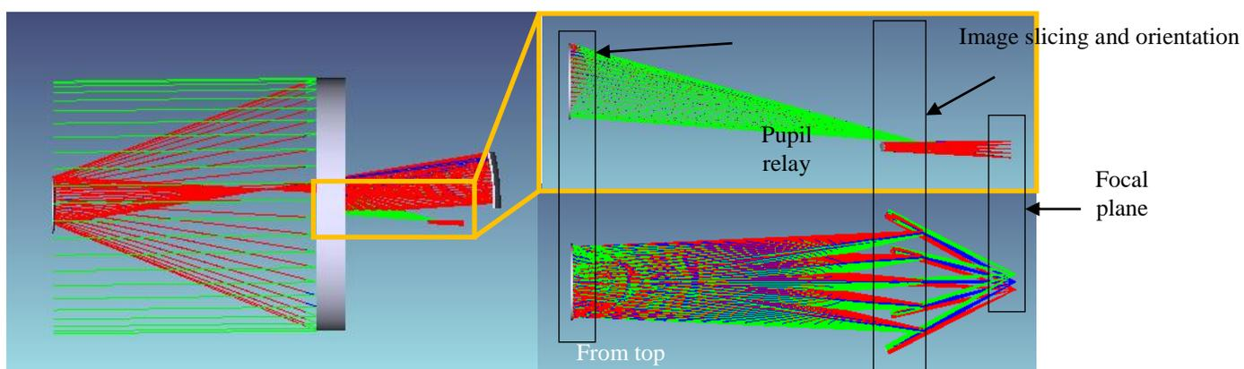
Fig. 4 Preliminary design of a Korsch F/5 telescope, with a 1.5m.
