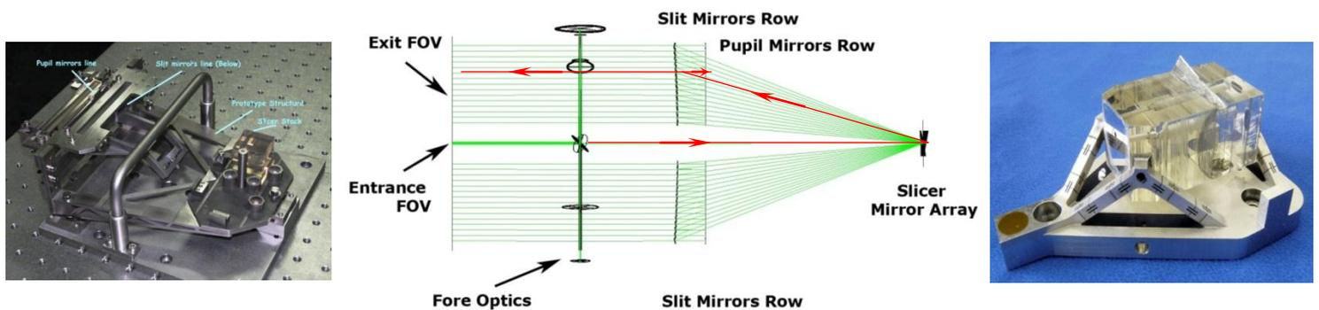
Fig.3 ESA prototype (2004, right) and qualification demonstrator (2006, left). Middle: optical design proposed for the NIRSpec instrument, managing tight positioning requirements.
