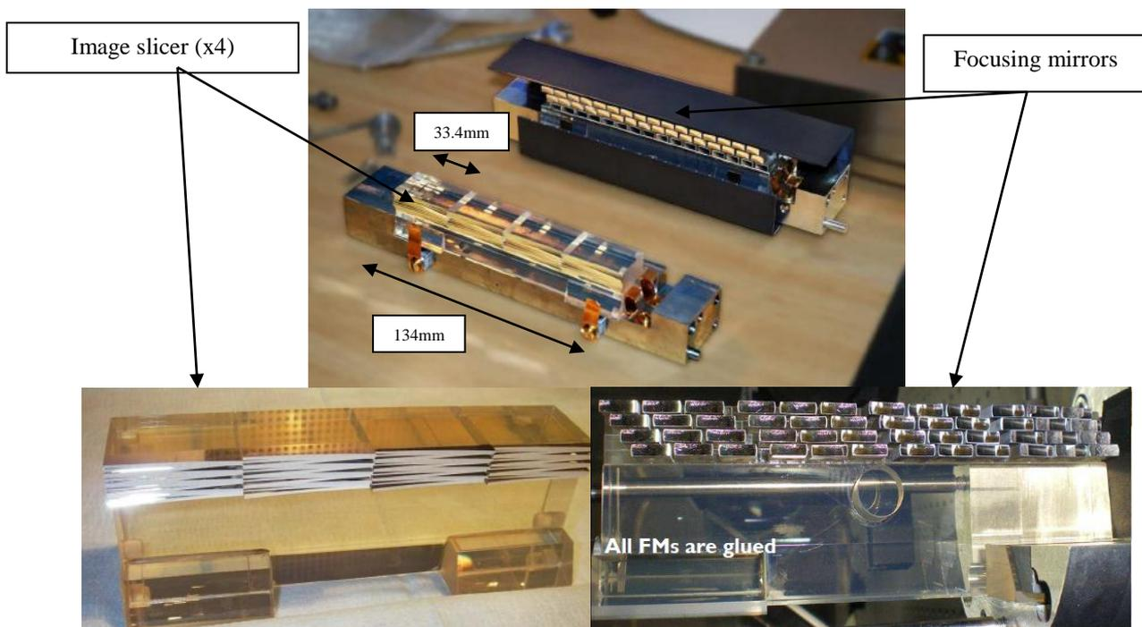
Fig. 2 A MUSE/VLT module made of four slicers and their associated focusing mirrors. (Credit ESO/CRAL/Winlight, Bacon et al 2012)
