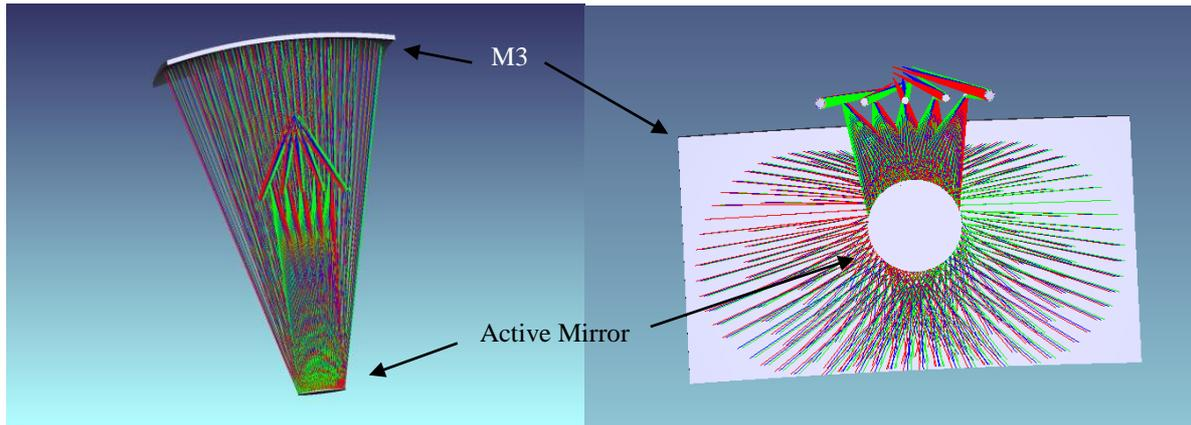
**Fig. 5 View of the focal plane module, including the tertiary mirror. The pupil relay can be used for active correction of the wave front.**
