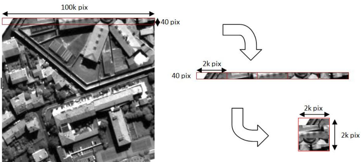
Fig. 1 schematic of reimaging a linear field over a 2D matrix
