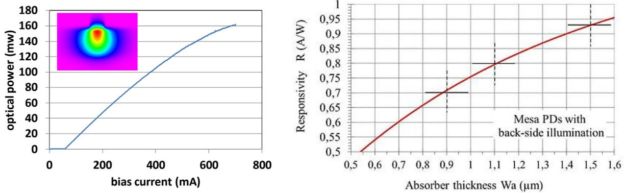
Fig. 2. (left) DFB experimental results from various devices within the 1<sup>st</sup> fabrication run and (right) simulation of the back-side illuminated UTC photodiode versus absorber thickness ( $W_a$ )
