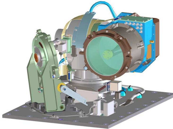
Figure 1 - Inertially Stabilized LLCD / LCRD Type Optical Module
