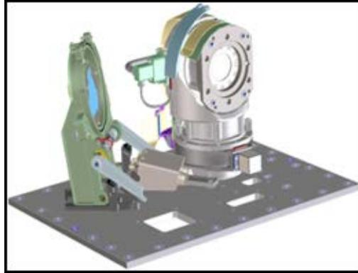
Figure 3 - Gimbal and Latch Assembly
